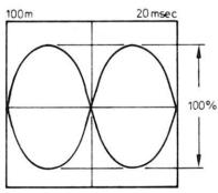
f) Loosen two securing screws and the move stepper motor on the basic frame so that the amplitudes show same illustration. Tighten motor securing screws (see figure)
